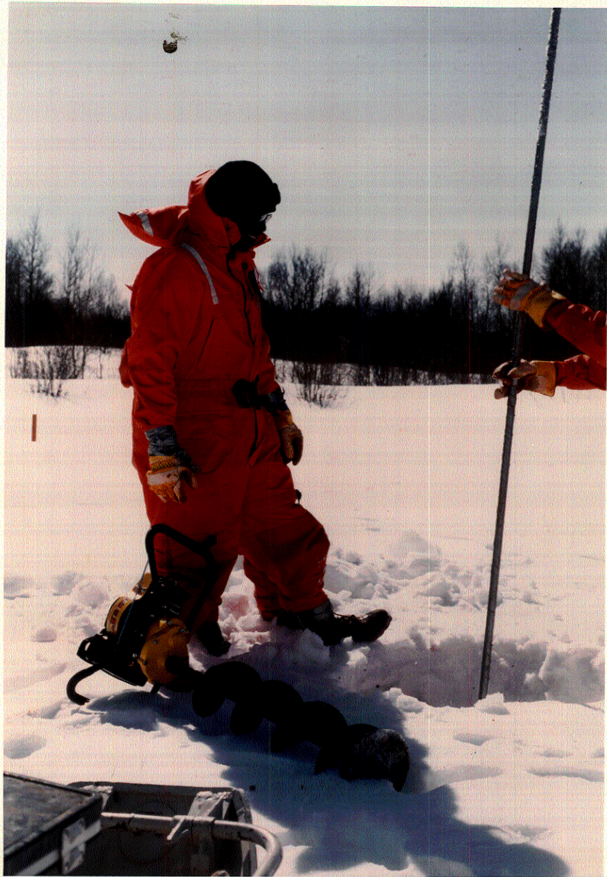
Figure 3: Winter sludge sampling using a hand corer.
